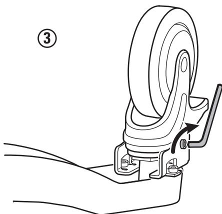
**Note:** Ensure that the wheel brakes face outward, away from the center column, when you slide on the brackets.
